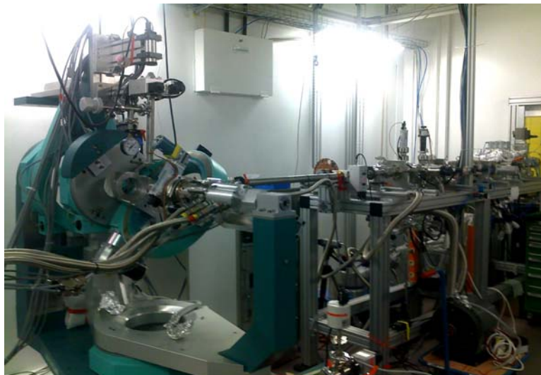
Fig. 3.14: An overview of the XAS experimental setup at BESSY. Two major parts are included, i.e. optical system of the beamline (right side) and detecting system of the fluorescence (left side).
